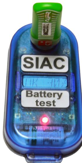
The station indicates sufficient battery reserve with a normal beep and a warning signal will sound if the battery is low. The battery check should be carried out in the event centre and not immediately before the start.
