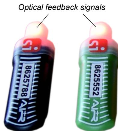
SIAC contains a battery and will always work in direct punching mode even if the battery is empty. Direct punching provides a fall-back option to register at controls. In contactless punching mode the SIAC's optical and acoustic feedback signals confirm that a control code and timestamp have been successfully written to the card.
