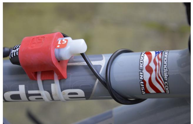
**WRONG** - Battery leads shall NOT be positioned by the SIAC
